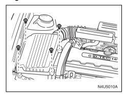
The engine air cleaner/filter is located on the passenger's side of the engine compartment. See "Engine Compartment Overview" in this section for more information on location.
